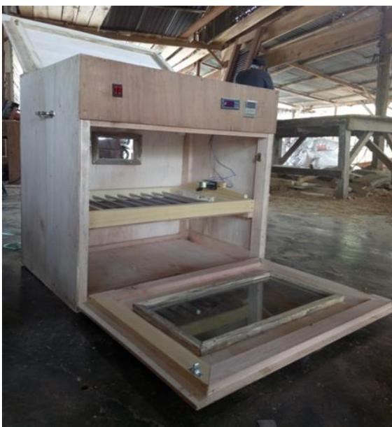
**Gambar 1.** Inkubator telur
